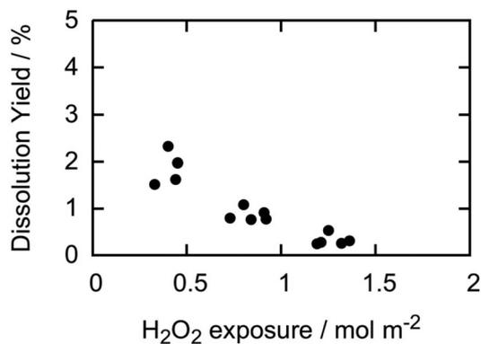
**Fig. 2** Dissolution yield vs. accumulated H<sub>2</sub>O<sub>2</sub> consumption per m<sup>2</sup> of exposed UO<sub>2</sub> for pellets in this study.
