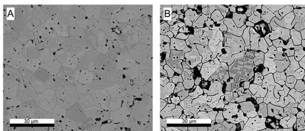
Fig. 4 BSE-SEM images of P3, (A) before the exposure to H<sub>2</sub>O<sub>2</sub> and (B) after the third exposure to H<sub>2</sub>O<sub>2</sub>.
