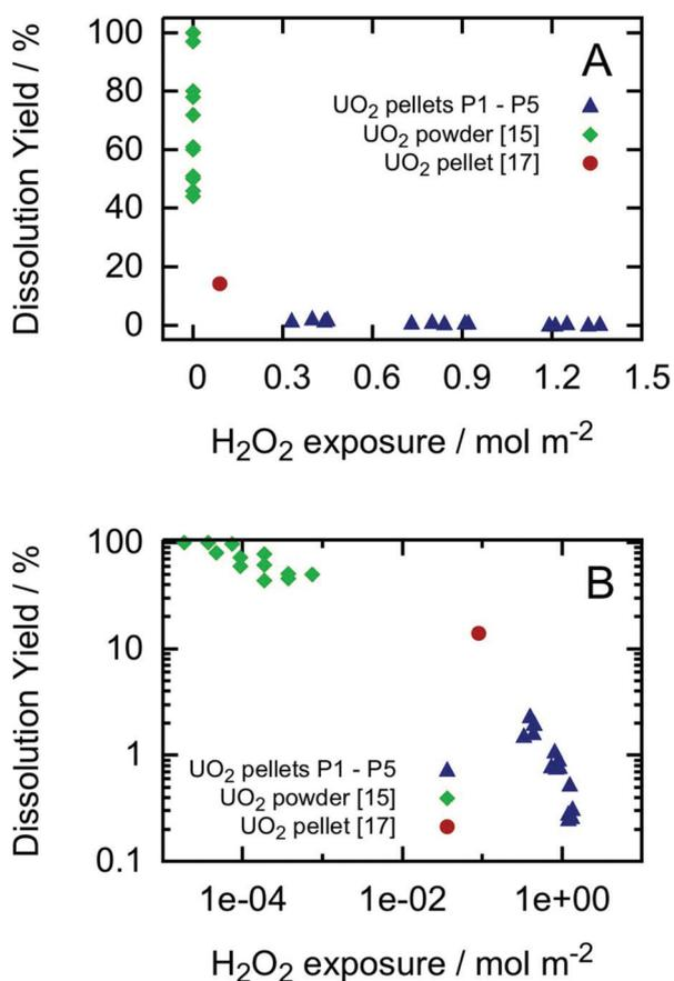
Fig. 3 Dissolution yield vs. accumulated H<sub>2</sub>O<sub>2</sub> consumption per m<sup>2</sup> of exposed UO<sub>2</sub>. UO<sub>2</sub> pellets from this study (blue triangles), UO<sub>2</sub> pellet<sup>20</sup> (red dot), as well as powders<sup>18</sup> (green diamonds). (A) Linear axes and (B) logarithmic axes.
