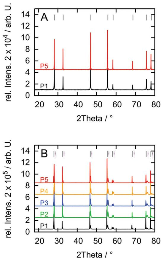
Fig. 6 (A) Diffractograms before the first  $\text{H}_2\text{O}_2$  exposure and (B) after the third  $\text{H}_2\text{O}_2$  exposure. Y-Axis offset is added for clarity. Indices for  $\text{UO}_2$  are shown as gray lines<sup>36</sup> and for  $\text{U}_4\text{O}_9$  as purple dashed lines.<sup>37</sup>
