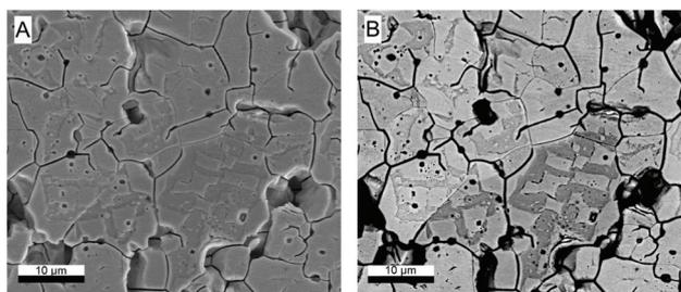
Fig. 5 (A) SE-SEM of P3 after the third exposure to H<sub>2</sub>O<sub>2</sub> and (B) BSE-SEM of the same area.
